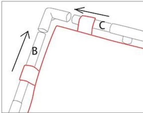
\* Put the hammock strap loops hanging on the upper plastic tubes while installing the upper frame
